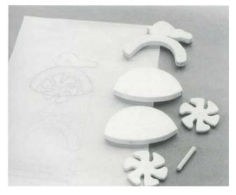
1 Check the component parts against the working draw ings. And just in case you are wondering why I opted to use two 1/4"" thicknesses to make up the 1/2"-thick spacer—rather than a single 1/2" thickness—the simple answer is that I had lots of pieces of 1/4" ply that needed to be used up.
