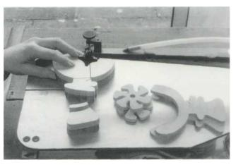
1 Having fitted the very finest blade in the scroll saw, very carefully cut the design down into its component parts. It's important that you use a new, well-tensioned blade and go at it slowly, so that each and every cut is well placed and square to the wood.
