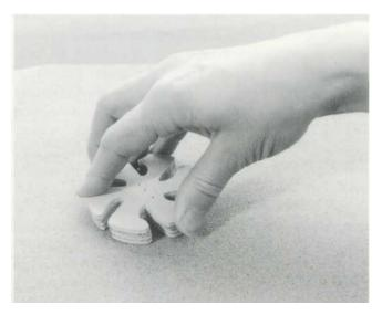
2 Fix the two wheels together with a piece of double-sided sticky tape and rub them down so that they are slightly less than 1/2" in total thickness. The use of the tape not only ensures that both wheels are identical, it also makes them easier to handle.
