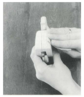
4 Rub the whole works down to a smooth finish. Close your eyes to test the finish—it's vital that every surface, edge and angle be supersmooth to the touch.
